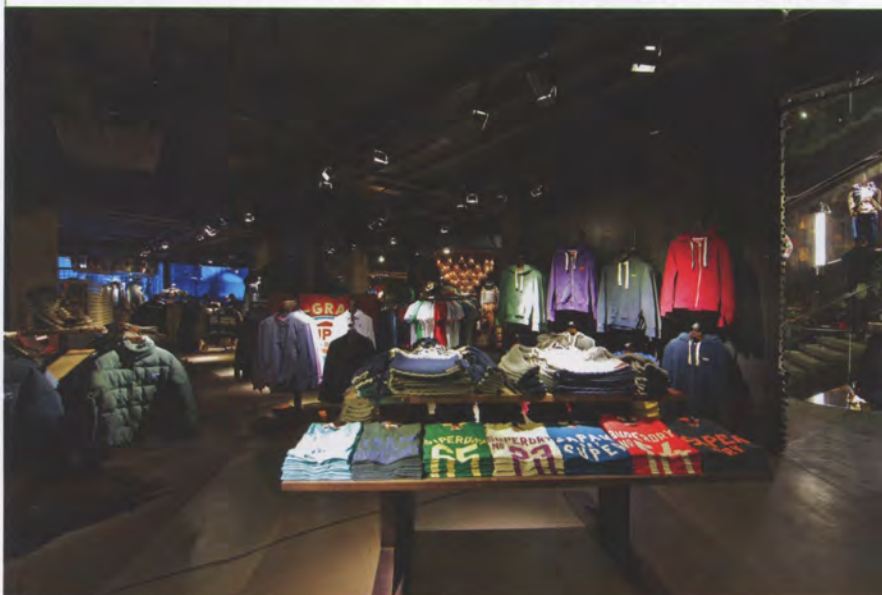
There is limited LED lighting in oval vitrine display cases (above) but most other lighting is provided by well-controlled, track-mounted metal halide spotlights (below)
