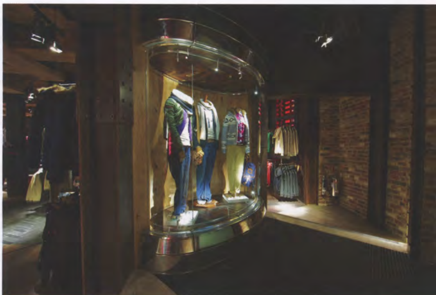
There is limited LED lighting in oval vitrine display cases (above) but most other lighting is provided by well-controlled, track-mounted metal halide spotlights (below)
