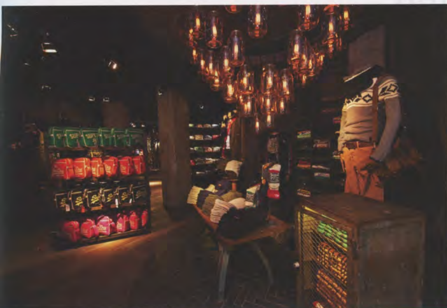
Dimmed down incandescent lighting is used in the quirky pendants, made from inverted glass jars as shades (above); and LED spotlights are integrated into the vertical shelving for close-up accent lighting (below).
