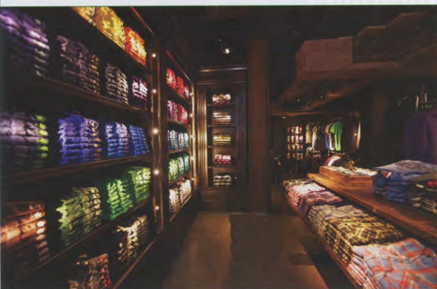
Dimmed down incandescent lighting is used in the quirky pendants, made from inverted glass jars as shades (above); and LED spotlights are integrated into the vertical shelving for close-up accent lighting (below).
