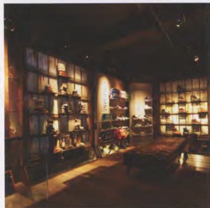
Metal halide spotlighting provides good vertical display illuminance to the merchandise
